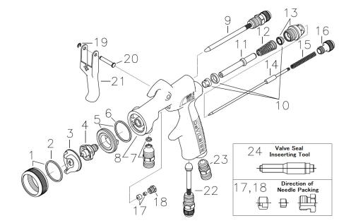
Note: Ref. No. 24 (LUNA2-34) is needed for Ref. No. 10 (LUNA2-443) installation. When removing it, be careful not to damage the surface of seat where inserted. A damaged seat may cause air leakage.
